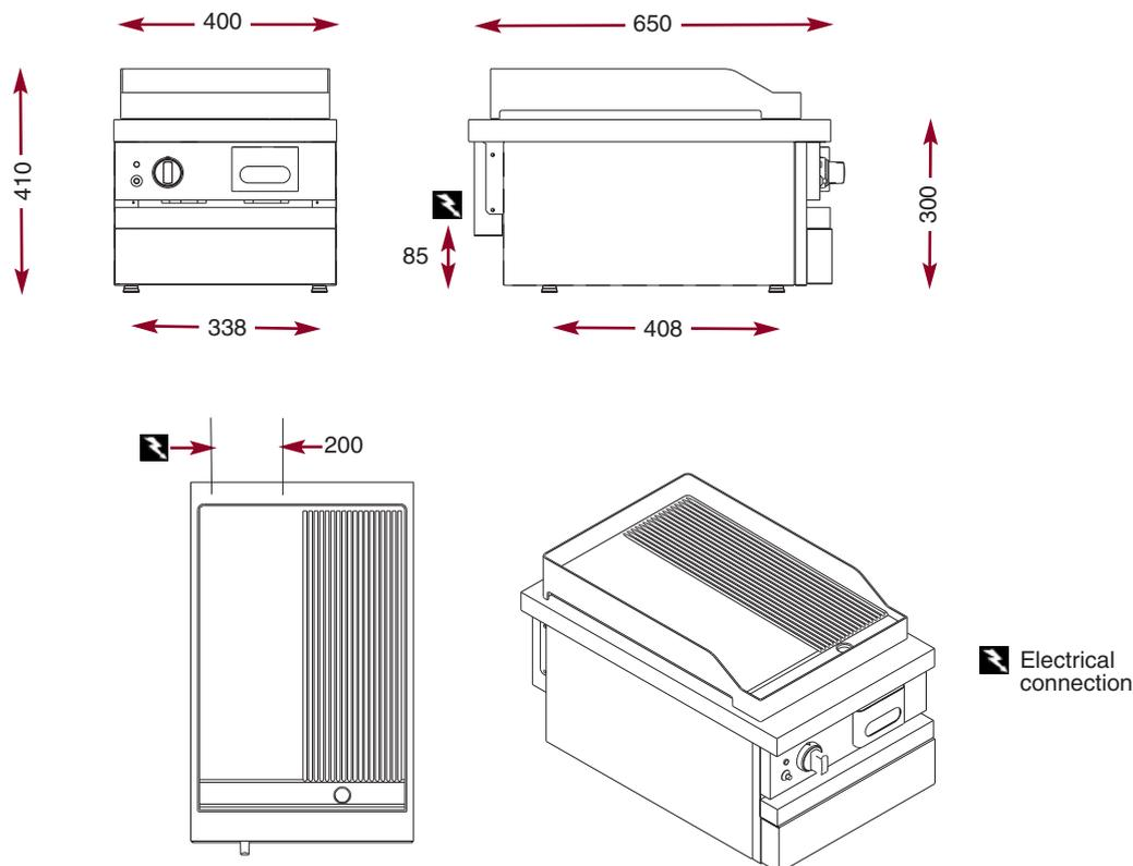
The modules have the same features and performances as the cupboard units. They are designed to be fixed onto tubular steel supports but can also be installed on stainless steel or tiled worktops.
